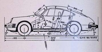
The specifications for overhang angles, curved and normal ground clearances apply to cars at full load.
