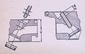
Machine 1st and 2nd oversize to correspond with bore in cylinder head. Press fit: 0.06–0.09 mm.
