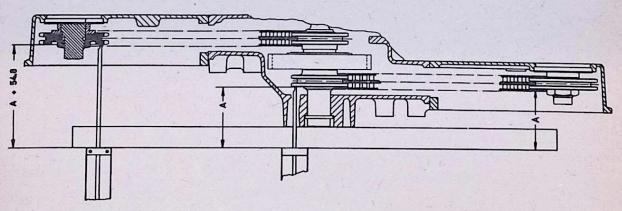
Example: measured dimension A = 78.7 mmThis means sprocket of cylinders 1 - 3 is A + 54.8 = 78.7 + 54.8 = 133.5 mm
